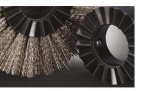
The Quick Snap is a true revolution in the area of disassembly. Thanks to the ingenious tooth pattern the brush segments are fastened together, which results in an even brush surface. Without the use of complicated tools you can quickly and easily assemble and dismantle (worn) brush segments within minutes and at any time. The Quick Snap brushes are fixed to the brush core by means of end collars. The brushes have been constructed as such that they can be used both left and right hand turned.
