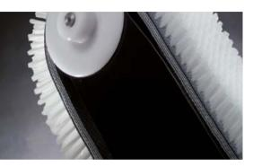
The core of a flat brush belt is made out of synthetic or chrome leather (CL). Chrome leather is the most used core material for the flat brush belt. Just as the V-string brush belt, the flat brush belt is used for applications such as transport and cleaning. The filling can be made from open to very dense which allows many different brush widths. By positioning the brush belt axially regarded to the product an optimal result is achieved.
