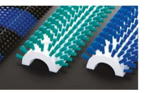
This type of roller brush is built up from two flexible split cores, which can be easily assembled on to the brush core. This system is mainly used for brushes that need to be changed often. Other brush cores can be difficult to dismantle.
